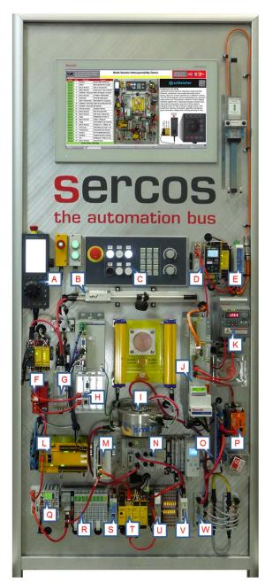
**P** The **KUNBUS** Gateway enables continuous and reliable communication between different networks and systems. The gateway converts all data that the target network can transfer. It omits non-transferrable data and adds necessary data in the new network. Thus, operators can transfer all necessary data from one closed network to another. The user can easily exchange the protocol modules to connect the Sercos automation bus to another network -Click & Plug & Play.
